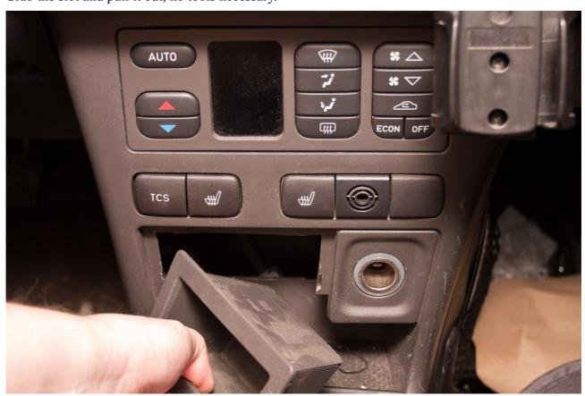
Push the buttons for tcs, and seat heating out from behind, then reach up and push the ACC panel out
